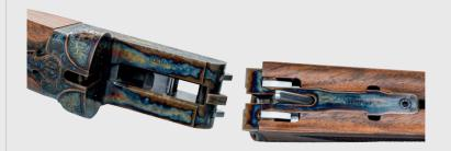
Holland & Holland type ejectors but with unbreakable coil springs and without vulnerable cocking lever sears
